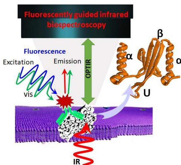
**Figure 1.** Schematic diagram of the working principle and lateral resolution for fluorescently guided optical photothermal infrared microspectroscopy.
