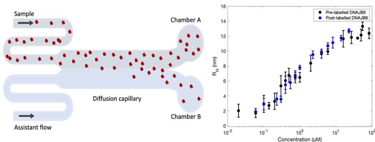
**Figure 1.** To the left: schematic of the MDS technique. Laminar flow of sample and assistant flow. Due to diffusion, some particles will end up in Chamber B. The portion of diffused particles reports on the mean hydrodynamic radius. To the right: DNAJB6b mean hydrodynamic radii at various protein concentrations (note the logarithmic scale), measured with MDS in both post- and pre-labeled set-ups.
